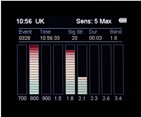
Live Cellular Mode showing three detected signals
