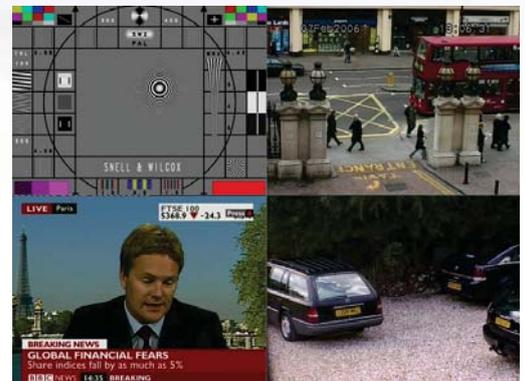
FourSight-DVI displays up to four PAL or NTSC images on one high resolution LCD display
