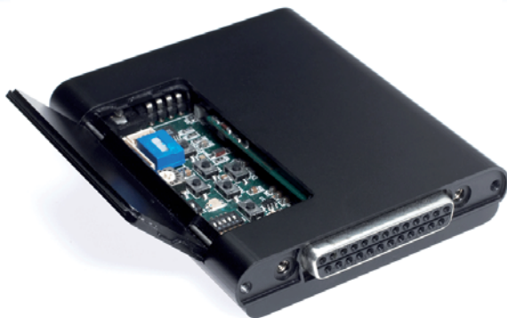
FlashBack-2 Motion Detector showing set up buttons and switches
